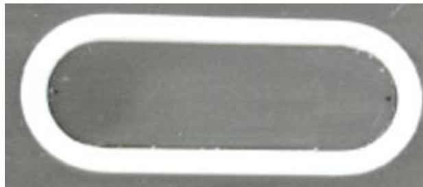
Figure 20. Active area of the \mu -PrepCell SS inlet block with Teflon O-ring.
