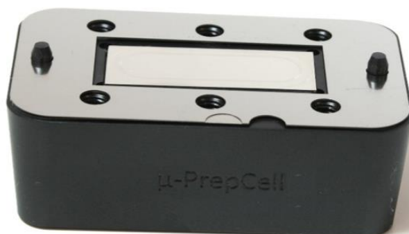
Figure 10. PEEK electrode block with Platinum electrode and stainless-steel spacers.
